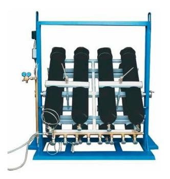
Plant for carbon dioxide gas feeding Additional equipment. "MINI".
