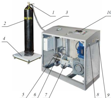
Carbon dioxide charging station SZU 800. General view.
